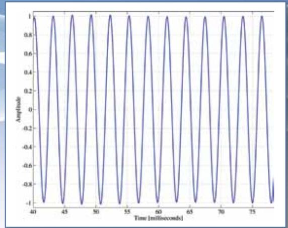
Figure 9: The result of applying the inverse transform to the spectrum in Figure 8c – a single sinusoidal wave.
