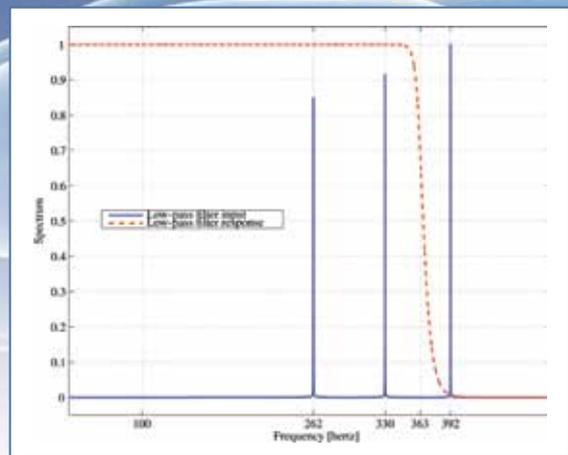
Figure 8a: The spectrum of the three-note chord with its low-pass filter response.
