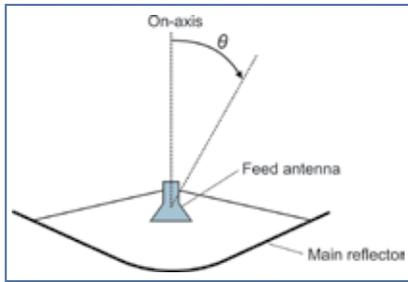
Figure 3: a (above): How electromagnetic waves are collected at the focal point of the parabolic reflector; b (right): The ideal gain pattern of a typical parabolic reflector antenna.
