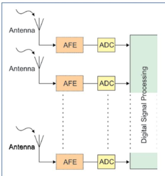
Figure 1: A simplified diagram of a general interferometer.
