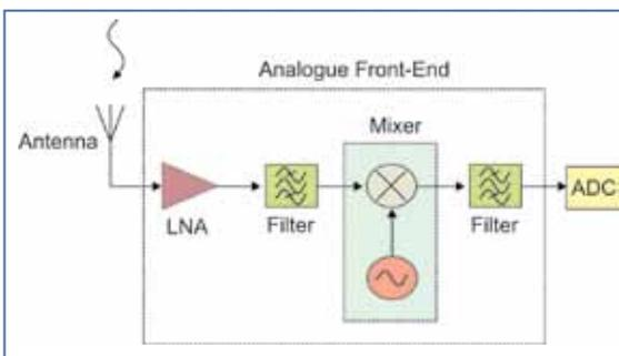
Figure 2: The components that make up the analogue front-end.
