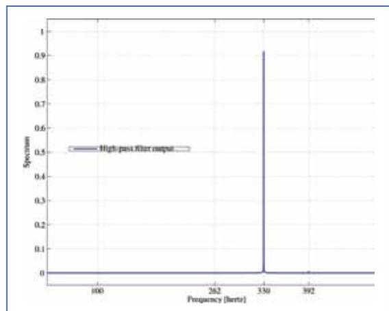
Figure 8c: The output of a high-pass filter – the lowest tone (262 Hz) has been removed from the signal so only E4 is left.
