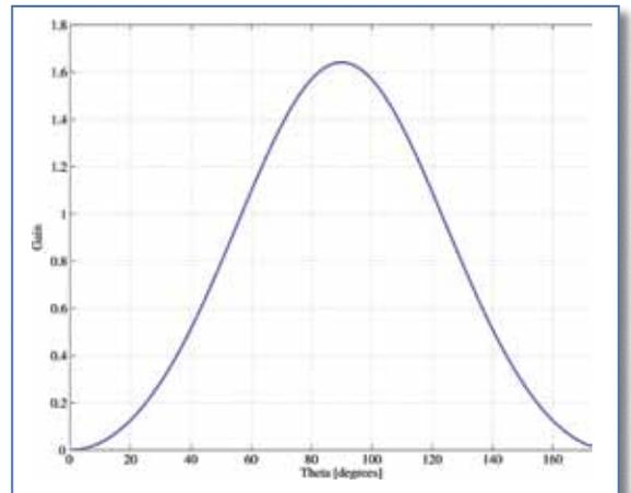
Figure 4: a (right): A dipole antenna; b (above): The radiation pattern of a single dipole antenna.
