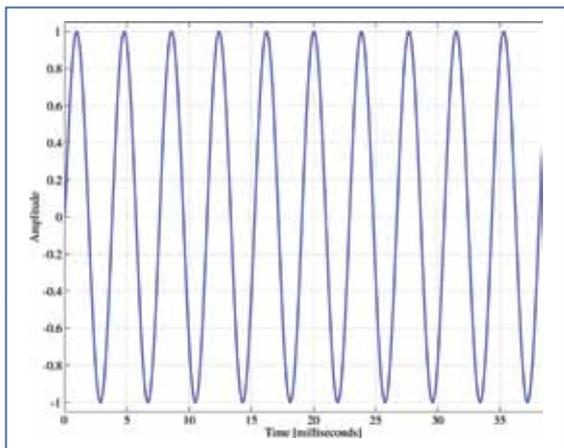
Figure 6a: The sinusoid produced when we plot the amplitude of a signal of 262 Hz as a function of time.
