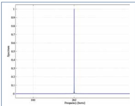
Figure 6b: The frequency spectrum of a signal of 262 Hz.
