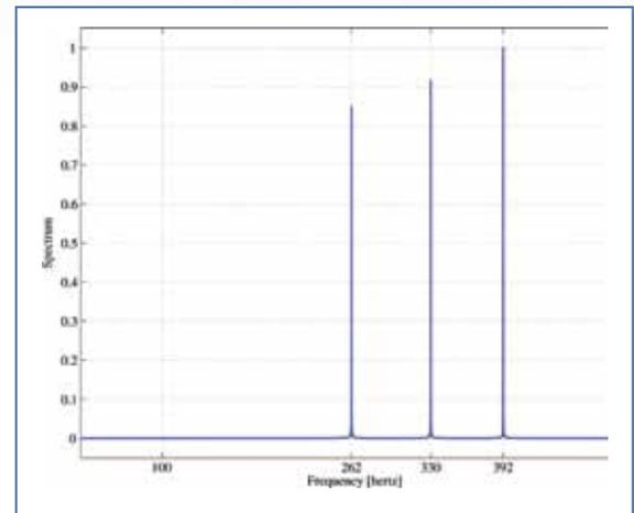
Figure 7: a (top): The signal produced by the three-note chord – C4, E4 and G4; b (above): The frequency spectrum of this signal.
