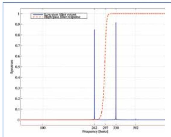
Figure 8b: The spectrum where the highest tone (392 Hz) has been removed, and the high-pass filter response.
