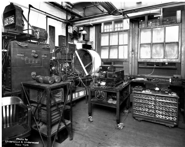
Fig. 7. Electronic laboratory at Western Electric, New York, c. 1915. The large inductor on the workbench was probably destined for the Arlington transmitter. Note trolleys containing a 90-V battery of dry cells and a mechanical oscillograph. Photograph from Vaal Teknorama.
