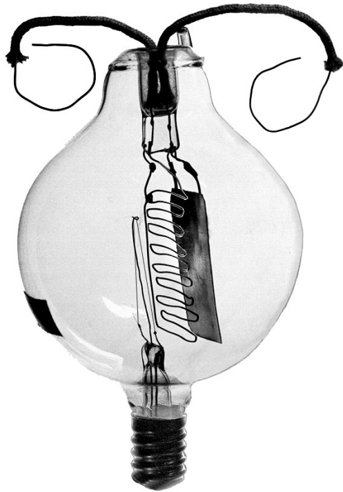
Fig. 6. A large anode de Forest Audion made especially for Western Electric for telephone repeater tests where higher power was required. The filament of this burnt out tube was added artificially. Tube in SAIEE collection; photo by the author.
